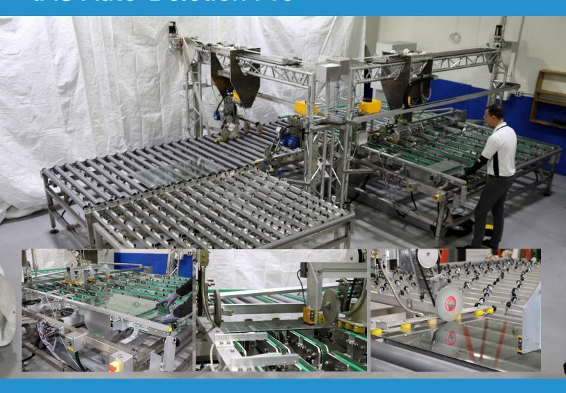
With the IAS Auto-Deletion Pro system, you load coated lites to the right. They pass under a deletion bridge with automatic glass-size sensing, turn left and pass under the second deletion bridge and then into the right-hand side of the washer.
