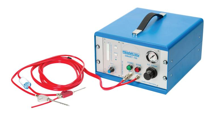
The HELANTEC SMART 150 has been developed for an economical gas filling process. The capacity is approximately 200 units per shift.
